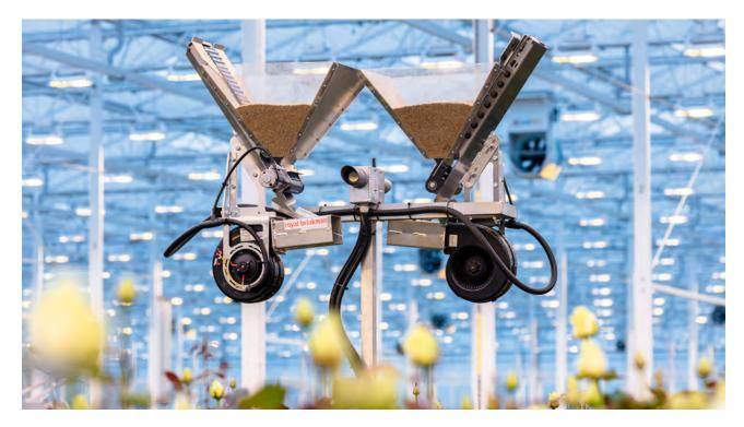
To create the widest possible, simple, fast and uniform distribution over the crop, the UniMite Air was developed. The UniMite Air is a bioblower system that combines simplicity and speed, enabling a maximum spreading width of 10 metres.
